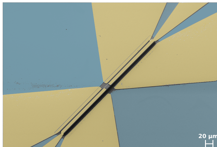
Figure 5.10: SEM picture of the finalized component before thinning and cleaving.
